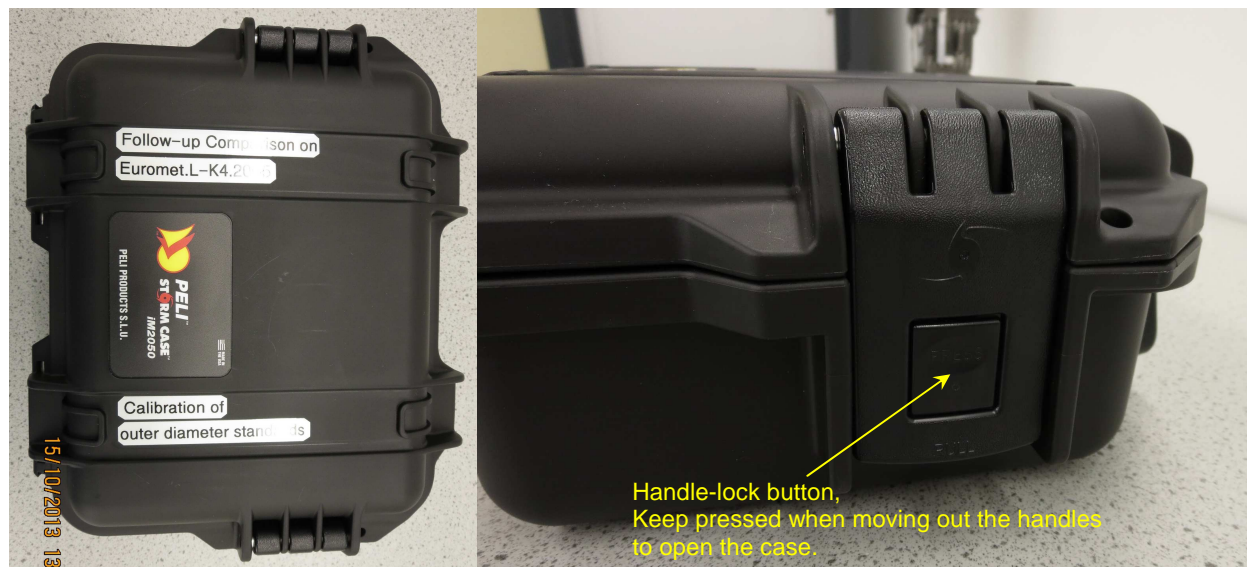
Figure 1: Air tight transportation case for the gauges
