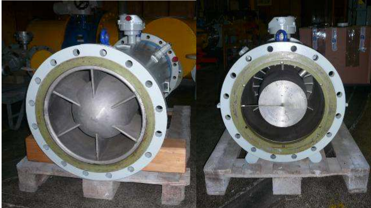
Figure 2 – Axial turbine gas meter ELSTER G6500
