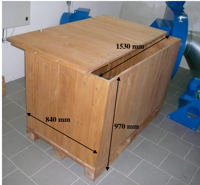
Figure 4 – The wooden box for the turbine gas meter G6500
