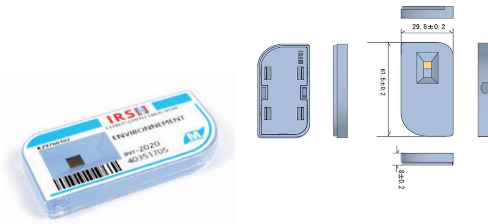
Figure 1 Passive RPL dosimeter provided by IRSN. The dimensions are approximately 29.8 mm x 61.5 mm x 8 mm.
