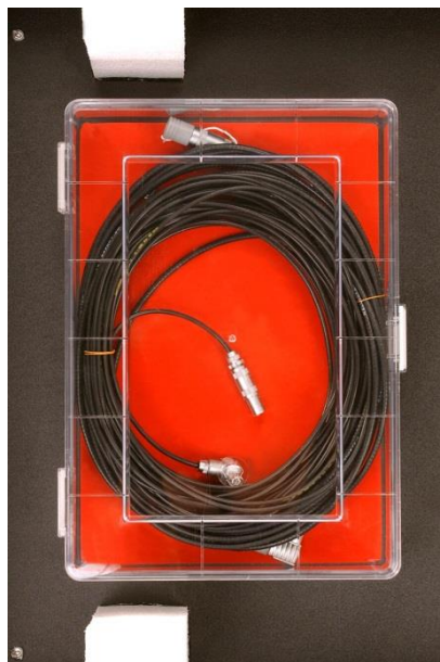
Figure 6: Cables stored in the front cover of the blue box: one cable for the chamber voltage and one for measuring the chamber current
