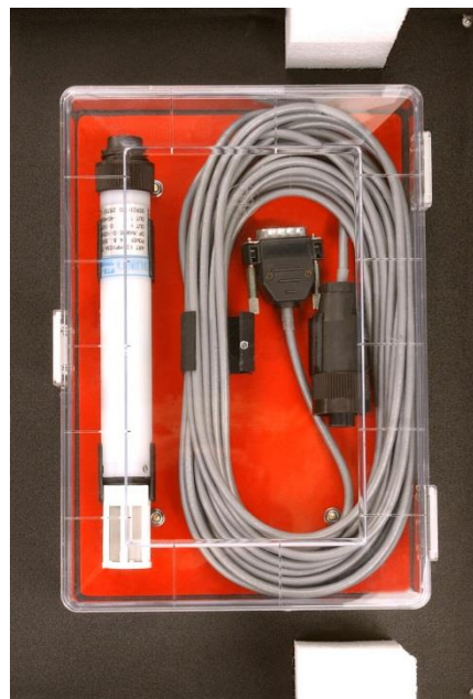
Figure 8: Sensor for measuring the temperature and rel. humidity together with its cable inside the front cover of the blue box.
