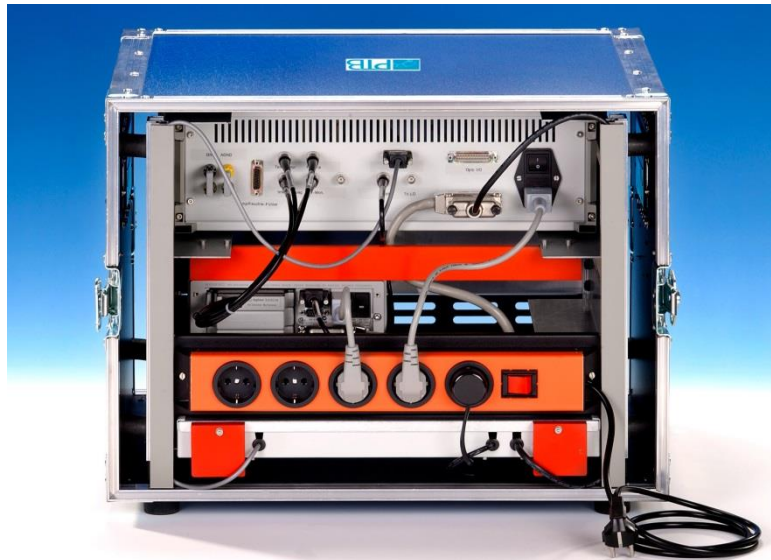
Figure 5: Back side of the electronic measuring device with distribution sockets and mains cable
