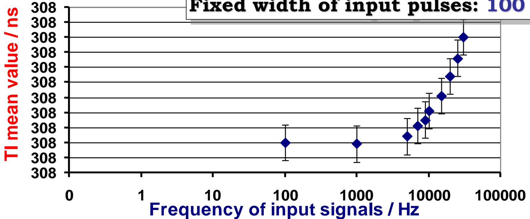
Up to about **5 kHz of input signal**, there is **no observed change of Time Interval between output signals of InLambda standard**
