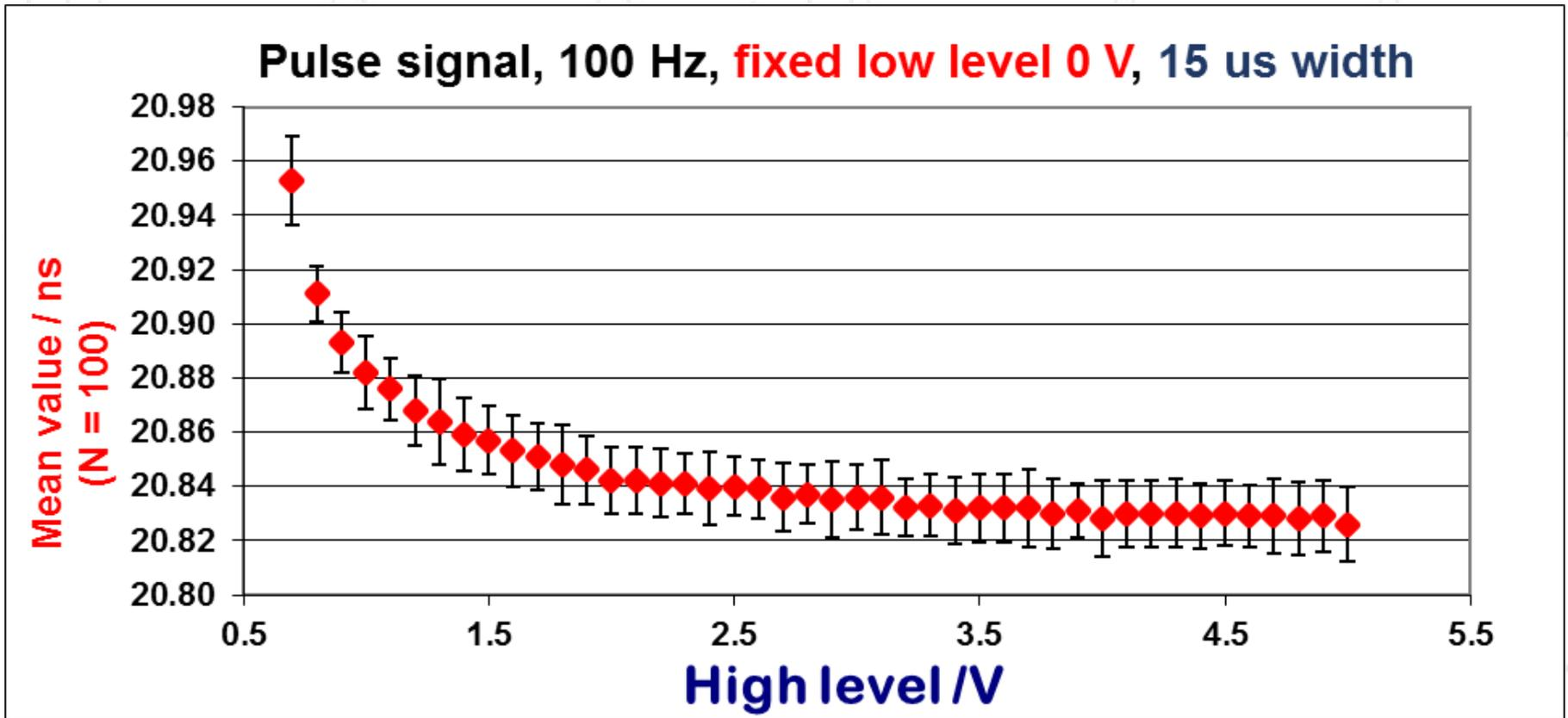
From about **2 V of the high level of input signal**, there is **slow change of Time Interval between output signals** with increasing the high level of input signal.
