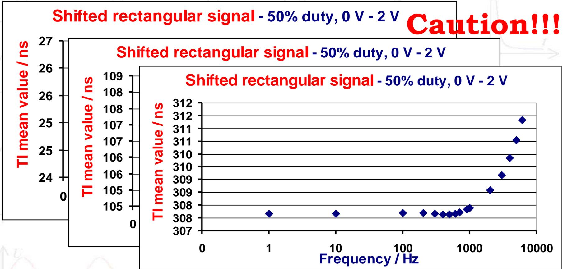
**Up to about 200 Hz of the shifted rectangular input signals (duty cycle 50%, low level 0 V, high level 2 V), there is no observed change of Time Interval between output signals.**
