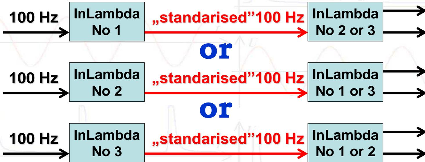
The problem of **the change of Time Interval between output signals** when the slope of input signals changes can be reduced by **the usage of the Start output signal of one InLambda standard to the input of the other InLambda standard** being measured.
