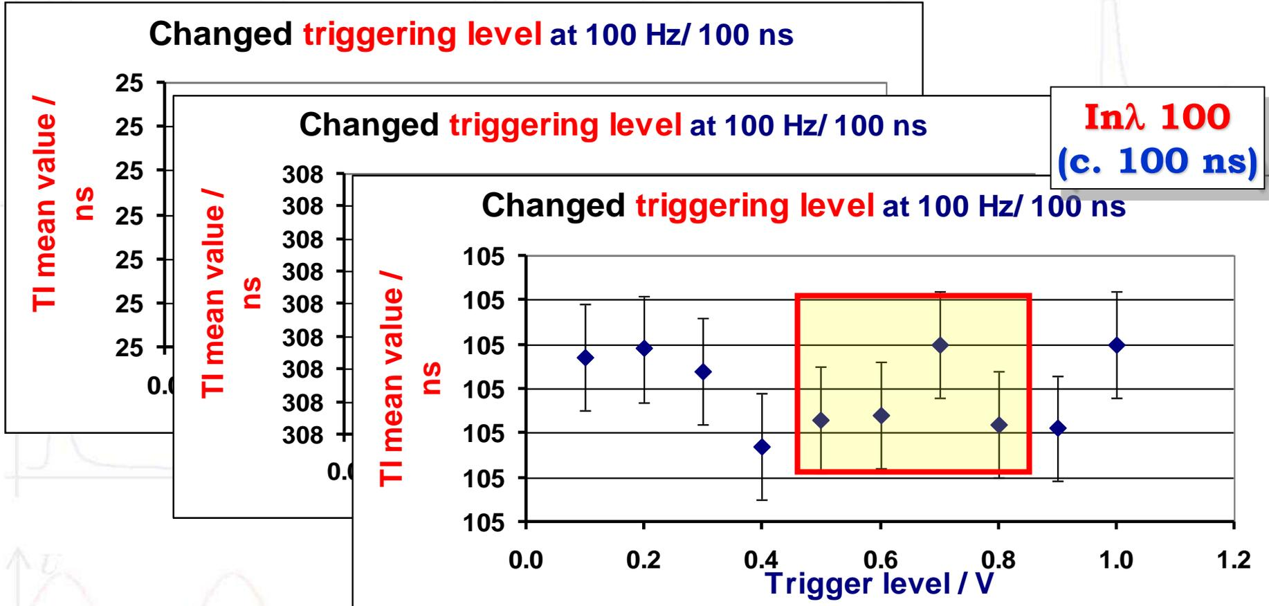
**It seems that 0.5 V or 0.6 V of the trigger levels would be better than 0.7 V**
