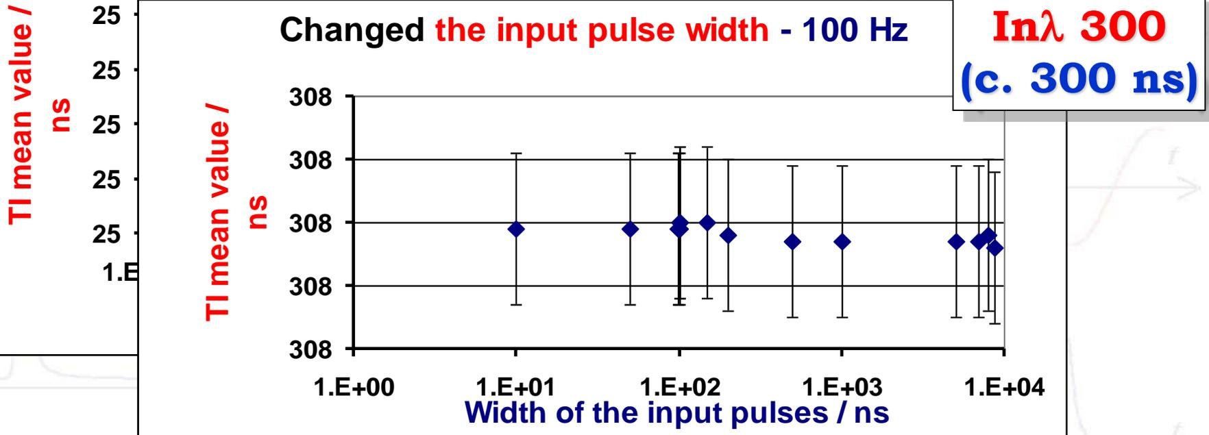
At frequency **100 Hz** of input signal, there is **no observed change of Time Interval between output signals** at least up to **9 ms** of the width of the pulses.
