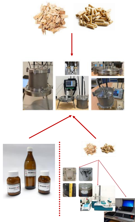
Figure 30: Illustration of traceability to the International System of Units (SI) achieved by using a secondary measurement standard calibrated with respect to a primary measurement standard or certified reference material for wood pellets or wood chips
