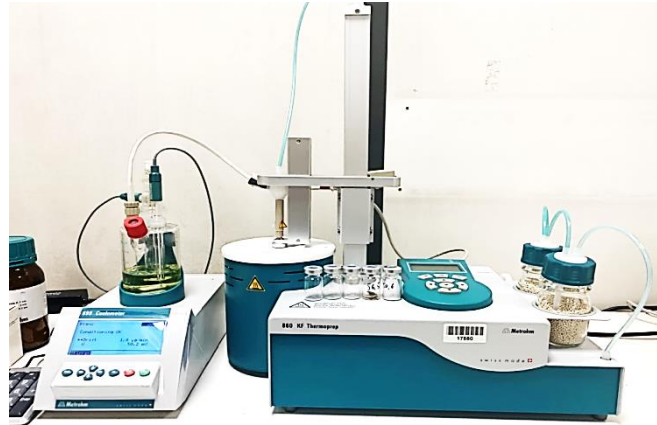
Figure 3 899 KF + 860 KF ThermoPrep for oven coulometric Karl Fisher titration – O-cKF or Evolved Water Vapour coulometric Karl Fischer titration
