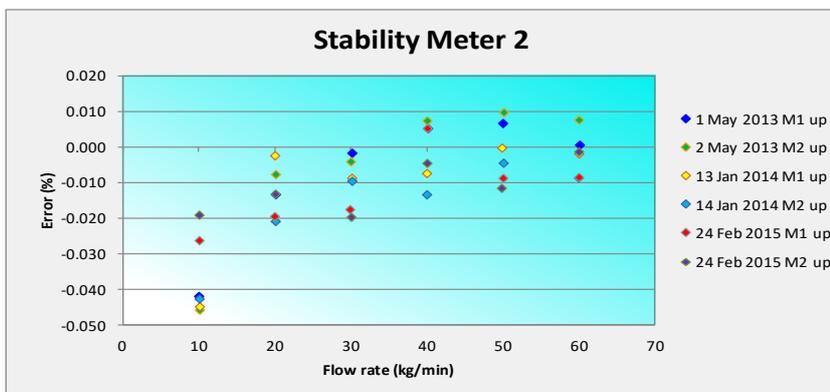
**Figure 7: Meter 2 Test results to determine the stability of the transfer standards**
