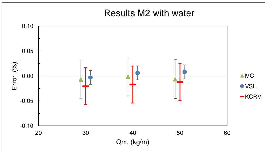
Figure 10: Meter 2 measurement error with uncertainty. (Error bars represent worst case for all rates.)
