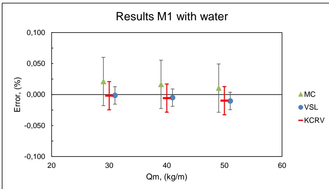
**Figure 8: Meter 1 measurement error with uncertainty. (Error bars represent worst case for all rates.)**
