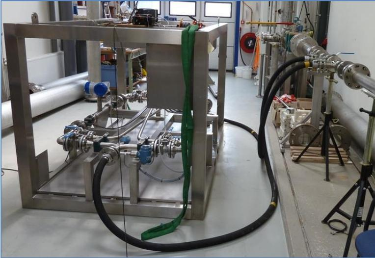
**Figure 1 - Picture of the IKS-SKID connected to a calibration facility (VSL Water Flow)**
