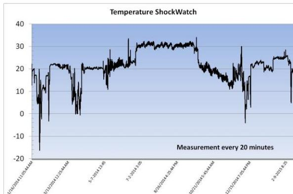
Figure 5 - Temperature registered by the ShockWatch® during the time of the comparison
