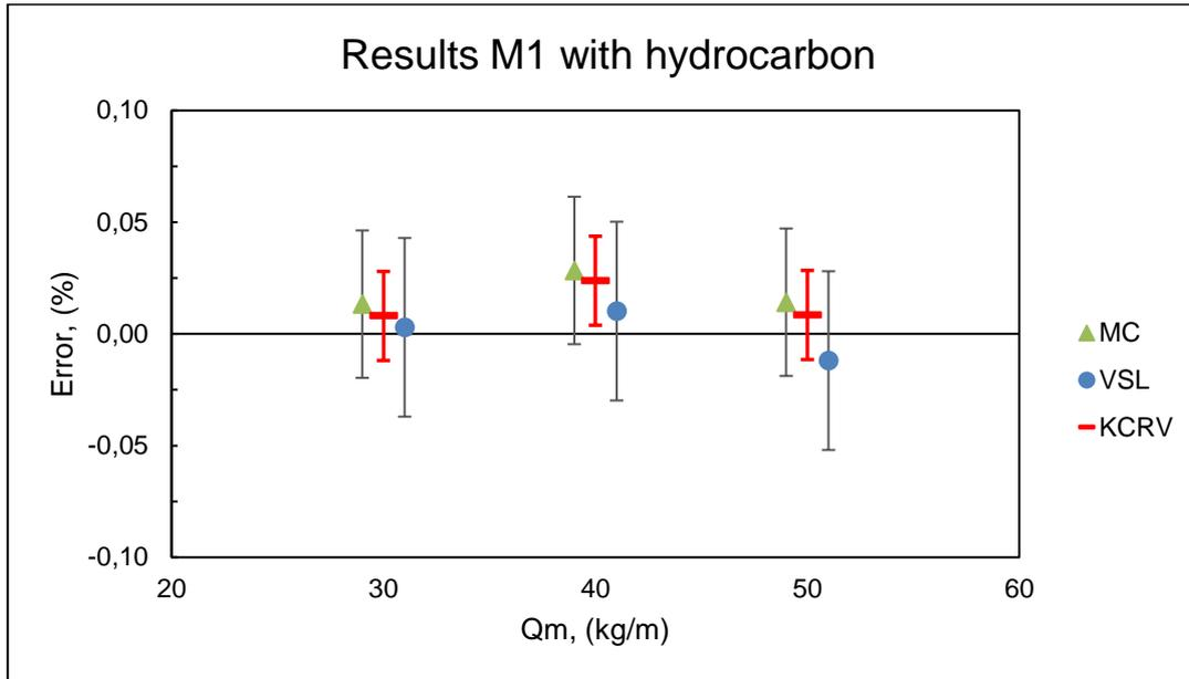
**Figure 12: Meter 1 measurement error with uncertainty. (Error bars represent worst case for all rates.)**
