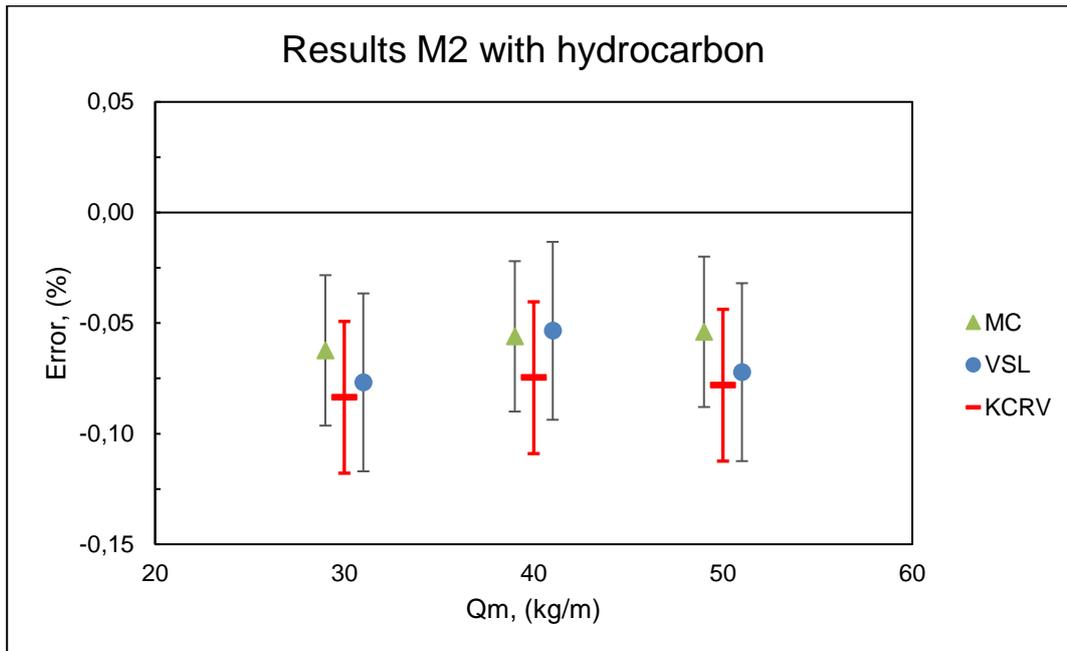
**Figure 14: Meter 2 measurement error with uncertainty. (Error bars represent worst case for all rates.)**
