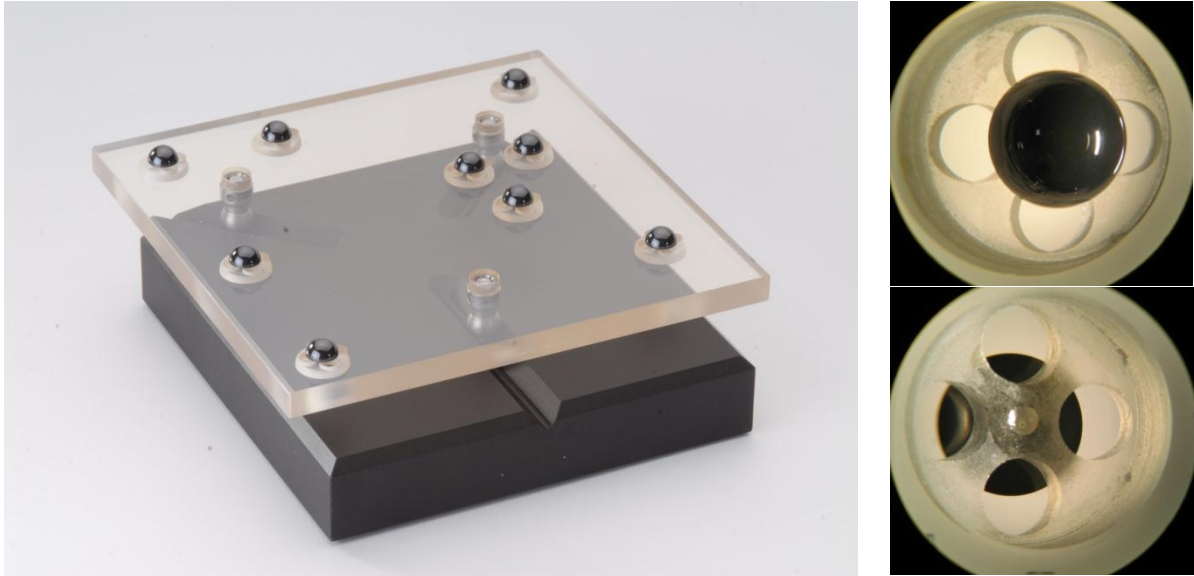
Figure 1. Zerodur plate with nine hemispheres, details: hemisphere top-side view and bottom-side view.
