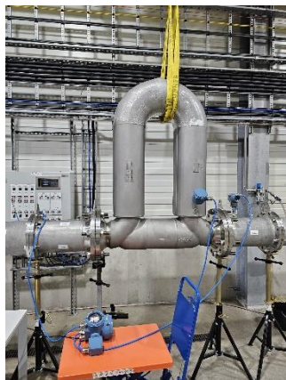
Picture 1 travelling standard and model 5700 transmitter.
