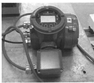
Installation of meter under test (MUT) in calibration line and transmitter of MUT
