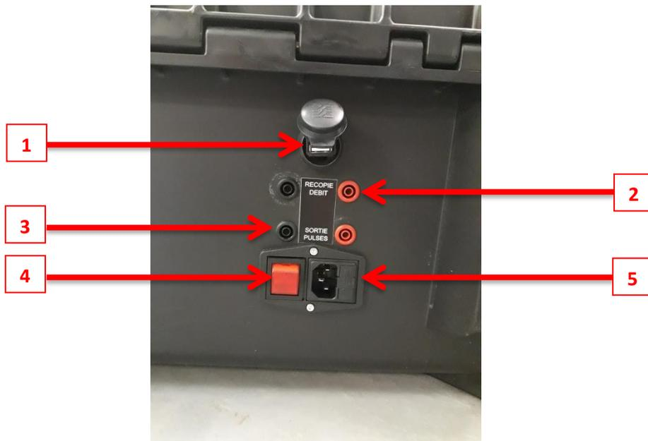
Figure 2: back side of the validation module
