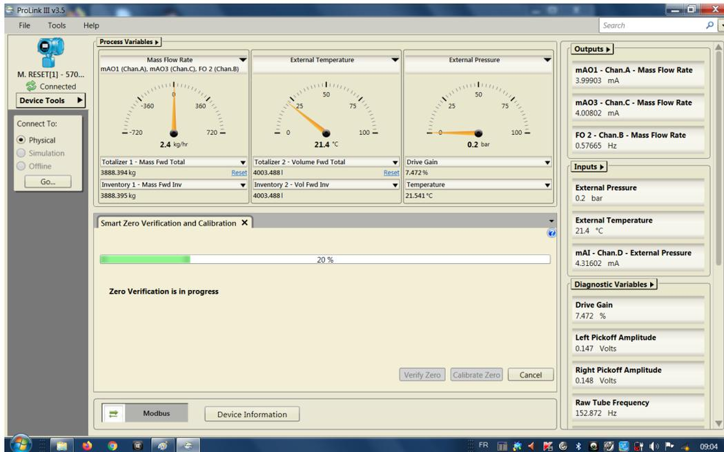
15. Click on "Calibrate Zero" to perform the zeroing of the meter as shown below.
