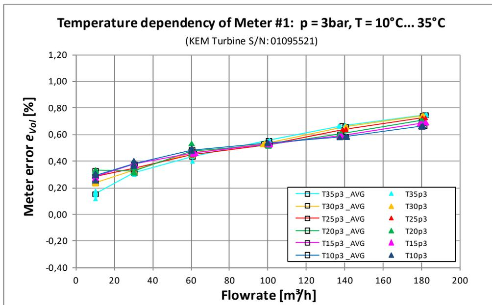
**Figure 13:** Temperature dependency of **Meter #1** (Turbine, KEM), measured at PTB in March and April 2013, fluid temperature: 10 °C, 15 °C, 20 °C, 25 °C, 30 °C and 35 °C, line pressure: 3 bar
