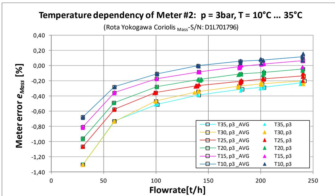
**Figure 15:** Temperature dependency of *Meter #2* (Coriolis<sub>Mass</sub>), measured at PTB in February and March 2012, fluid temperature: 10 °C, 15 °C, 20 °C, 25 °C, 30 °C and 35 °C, line pressure: 3 bar.
