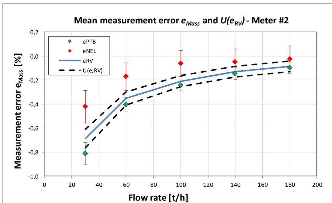
**Figure 36:** Measurement error of  $\bar{e}_{Vol}$  with error bars  $U(\bar{e}_{Mass})$  for PTB and NEL of **Meter #2**. reference value  $e_{RV}$  and the area of the extended uncertainty of the reference value  $U(e_{RV})$  – for **Meter #2**
