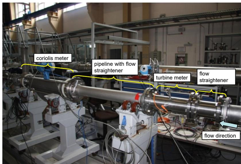
**Figure 2:** View on the transfer standard package at PTB test field (setup in May 2013)
