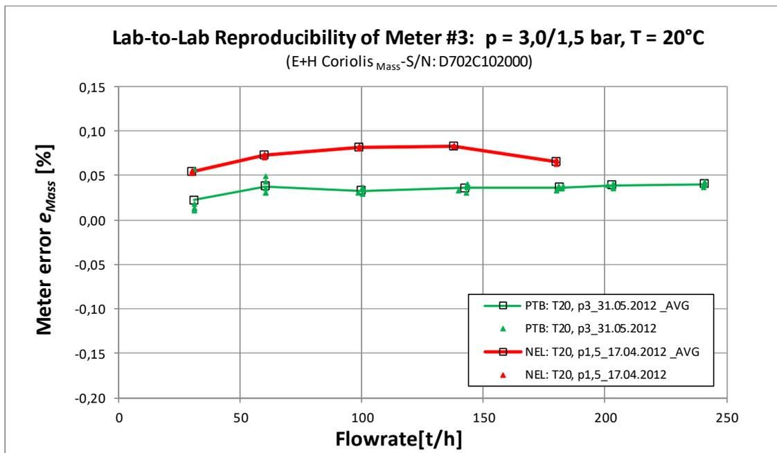
**Figure 31:** Lab-to-Lab Reproducibility of **Meter #3**, measured at PTB on 31.05.2012 and at NEL on 17.04.2012. Fluid temperature 20°C (both at PTB and NEL), line pressure: 3.0 bar at PTB and 1.5 bar at NEL. K-factor: 50 pulses/kg (both at NEL and PTB).
