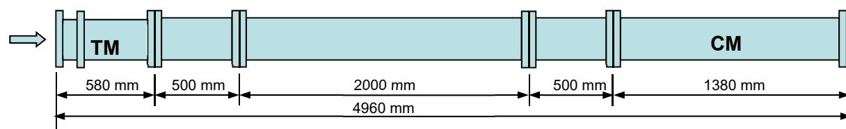
**Figure 1:** Schematic of transfer standard package (flow from left to right)
