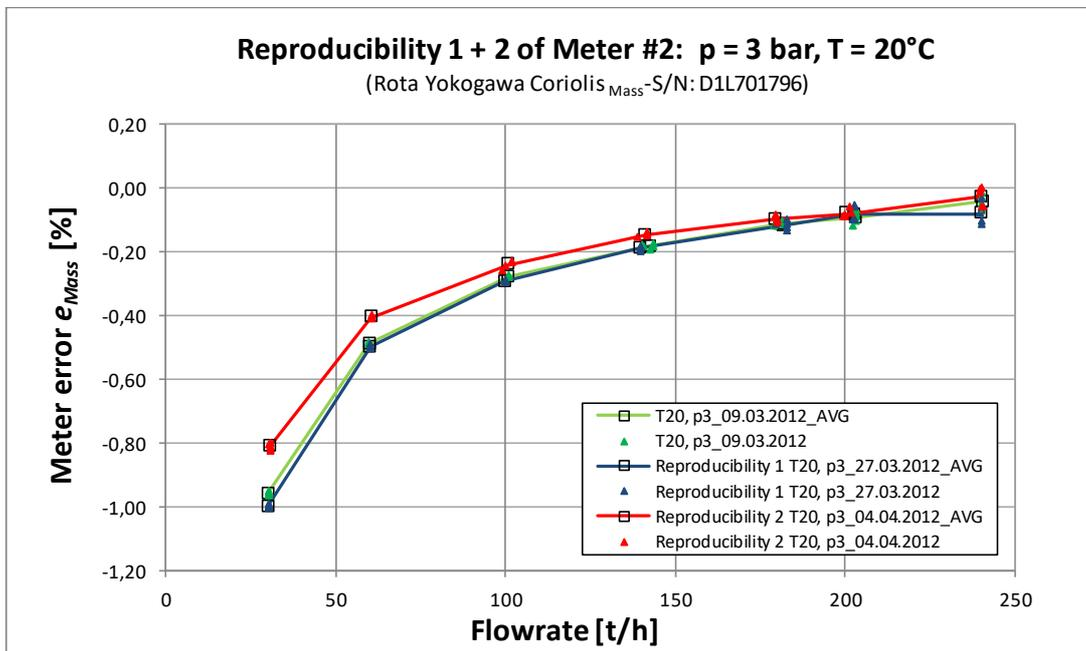
**Figure 23:** Internal reproducibility 1 and 2 of **Meter #2** (Coriolis<sub>Mass</sub>, Rota Yokogawa - S/N: D1L701796) measured at PTB in March and April 2013, line pressure: 3 bar, fluid temperature: 20 °C.
