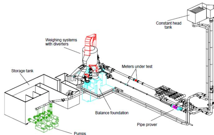
**Figure 10:** Cut-away view of PTB's water flow calibration facility
