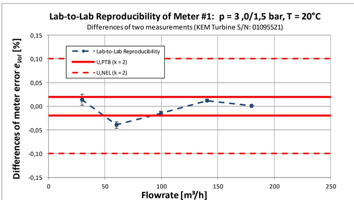
**Figure 28:** Lab-to-Lab reproducibility of **Meter #1** - Differences of measurement error data (25.04.2012 vs. 31.05.2012) of Figure 27 including error bars of maximum standard deviation for one of the comparison pairs
