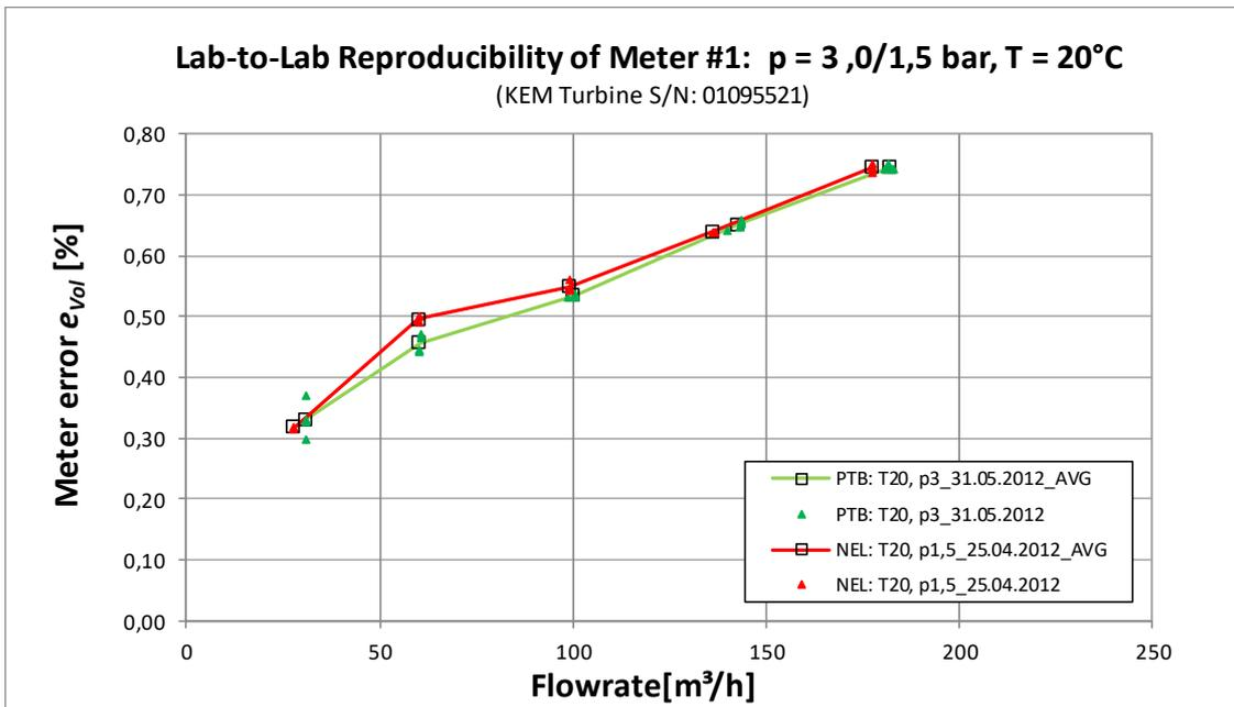
**Figure 27:** Lab-to-Lab reproducibility of **Meter #1**, measured at PTB on 31.05.2012 and at NEL on 25.04.2012. Fluid temperature 20 °C (both at PTB and NEL), line pressure: 3,0 bar at PTB and 1,5 bar at NEL. K-factor: 6,633 pulses/l (both at PTB and NEL)
