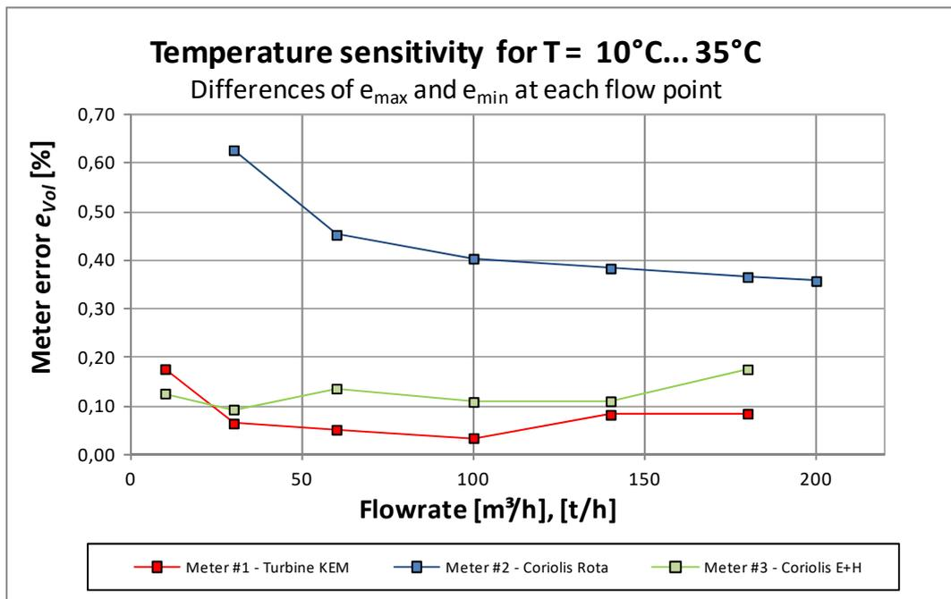
**Figure 20:** Temperature sensitivities of Meter #1, #2 and #3: differences of maximum and minimum  $\bar{e}$  for the fluid temperature range of 10 °C, 15 °C, 20 °C, 25 °C, 30 °C and 35 °C at each flow point, measured at PTB in March and April 2013, line pressure: 3 bar.
