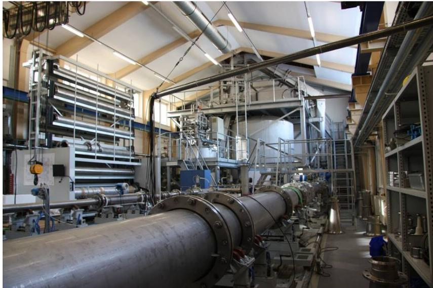
**Figure 9:** Water flow calibration facility at PTB
