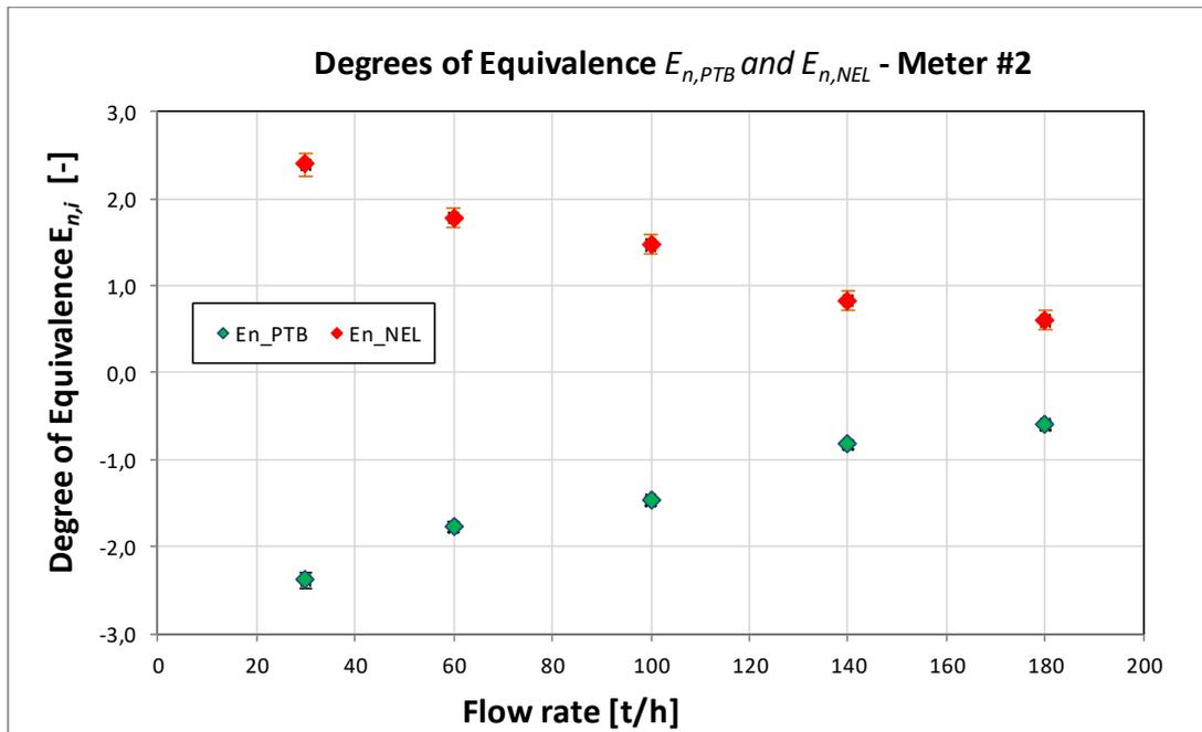
**Figure 35:** Degrees of equivalence  $E_{N,PTB}$  and  $E_{n,NEL}$  of **Meter #2** with error bars of  $u_{e,PTB}$ , respectively  $u_{e,NEL}$
