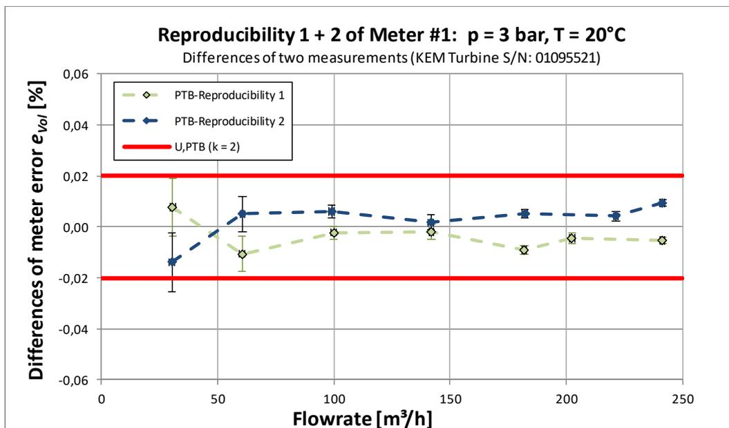
**Figure 22:** Internal reproducibility 1 and 2 of **Meter #1** - Differences of measurement error  $e_{Vol}$  for repeatability data (07.06.2012 vs. 31.05.2012) and for reproducibility data (11.06.2012 vs. 07.06.2012) of Figure 21 including error bars of maximum standard deviation for one of each pairs
