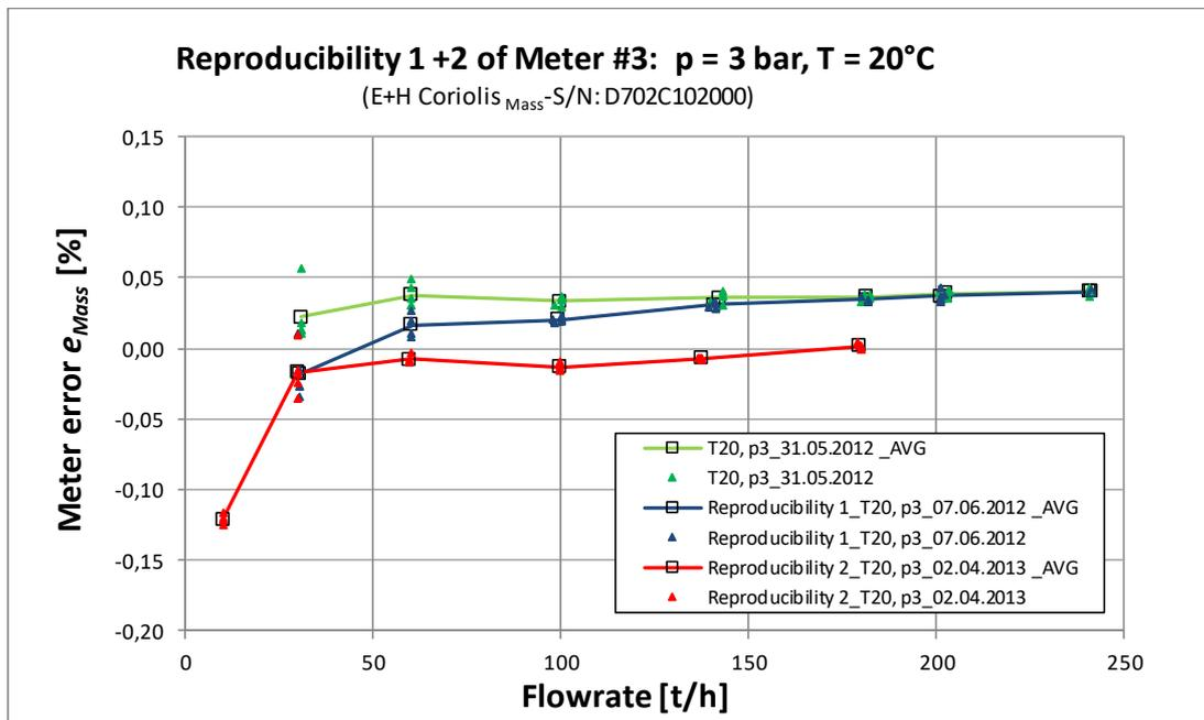
**Figure 25:** Internal reproducibility 1 and 2 of **Meter #3** (Coriolis<sub>Mass</sub>, Endress+Hauser - S/N: D702C102000) measured at PTB in May/June 2012 and March 2013, line pressure: 3 bar, fluid temperature: 20 °C.
