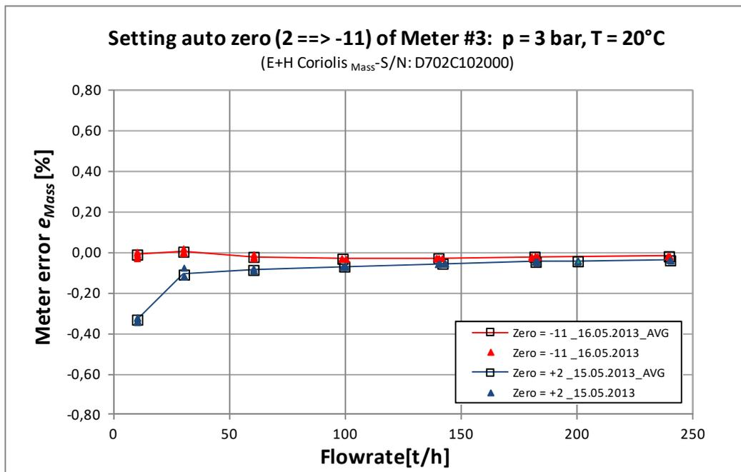
**Figure 19:** Influence of setting zero point from “+2” to auto zero value “-11” of Meter #3, measured at PTB in May 2013, line pressure: 3 bar, fluid temperature: 20 °C.
