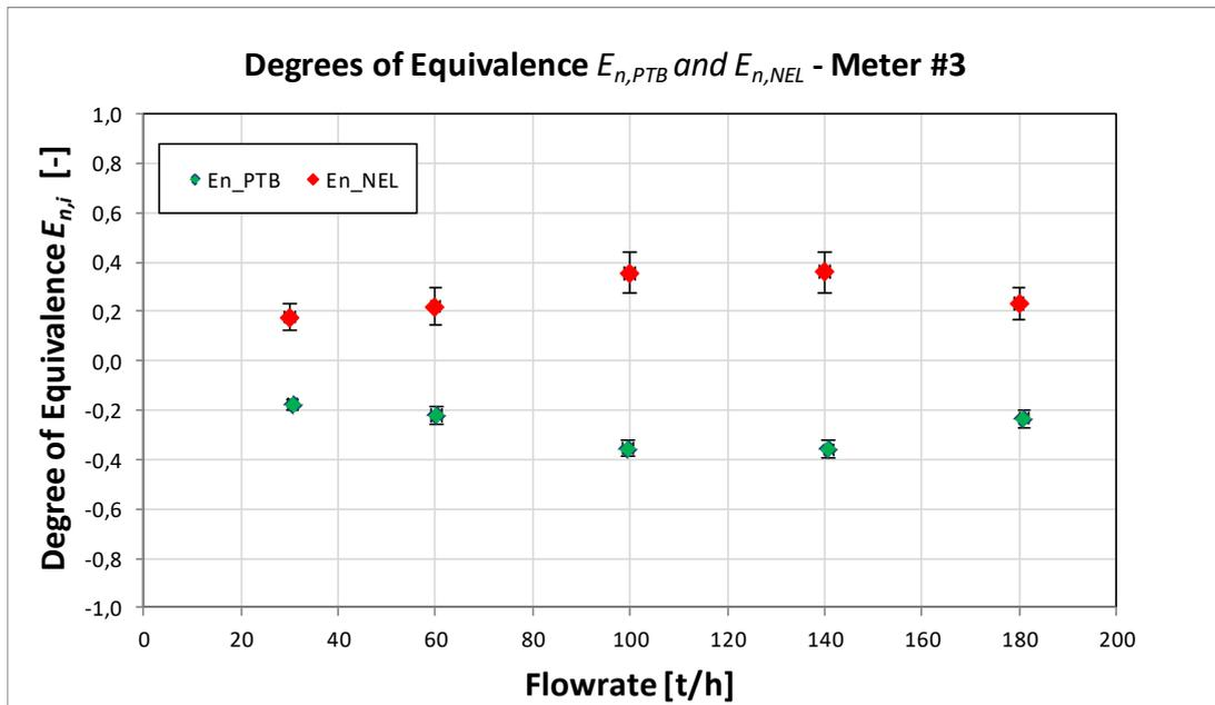
**Figure 37:** Degrees of equivalence  $E_{n,PTB}$  and  $E_{n,NEL}$  of **Meter #3** with error bars of  $u_{e,PTB}$  respectively  $u_{e,NEL}$
