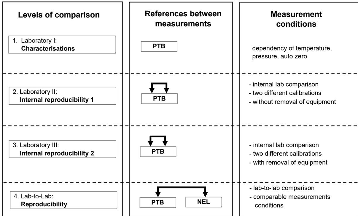
**Figure 12:** Practiced evaluation procedure of the four comparison stages
