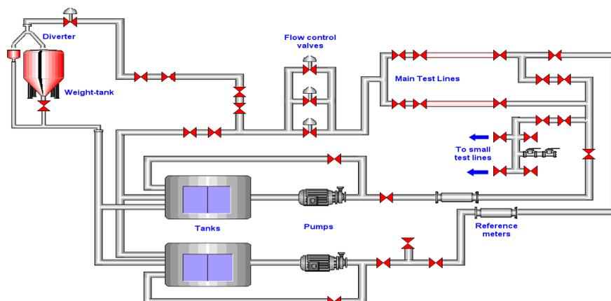
**Figure 7:** Schematic of NEL's water flow calibration facility.
