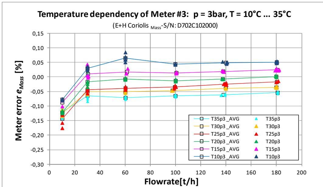
**Figure 17:** Temperature dependency of **Meter #3** (Coriolis<sub>Mass</sub>), measured at PTB in March and April 2013, fluid temperature: 10 °C, 15 °C, 20 °C, 25 °C, 30 °C and 35 °C, line pressure: 3 bar.
