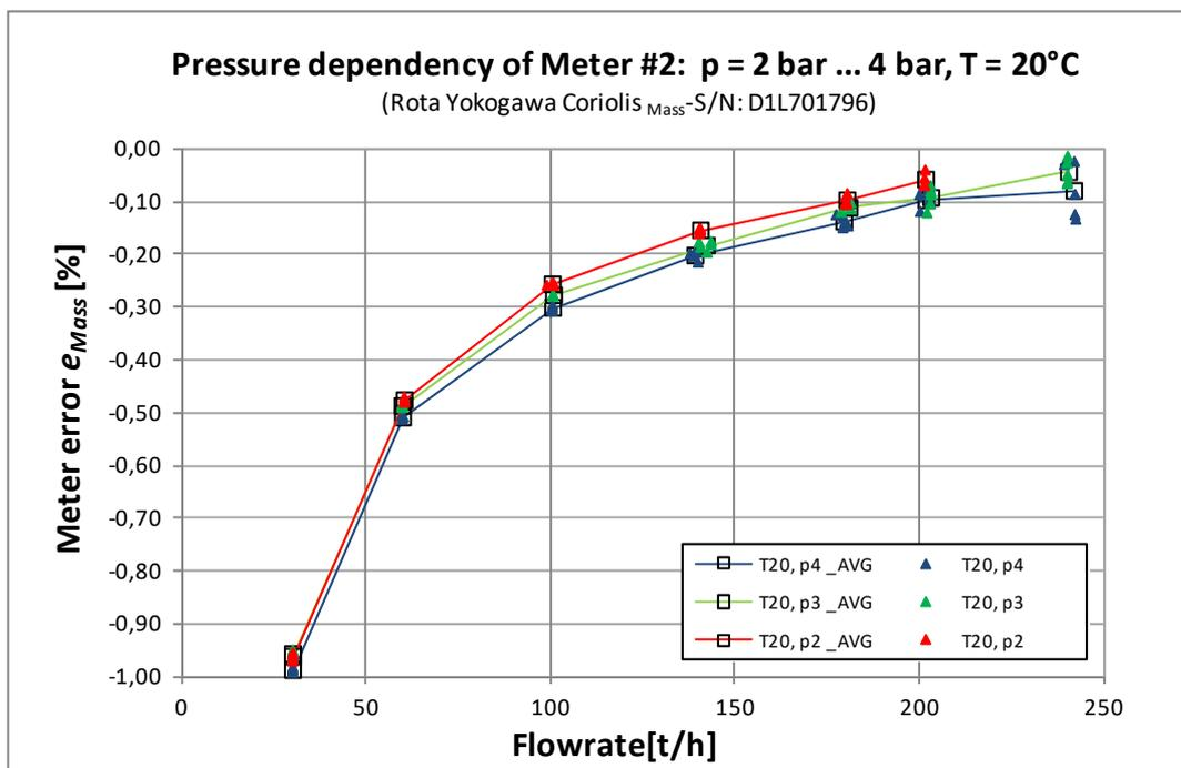
**Figure 16:** Pressure dependency of *Meter #2* (Coriolis<sub>Mass</sub>), measured at PTB in March 2012, line pressure: 2 bar, 3 bar and 4 bar, fluid temperature: 20 °C.
