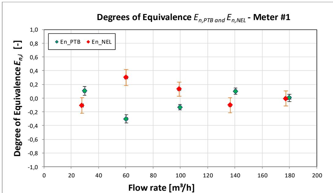
**Figure 33:** Degrees of equivalence  $E_{n,PTB}$  and  $E_{n,NEL}$  of **Meter #1** with error bars of  $u_{e,PTB}$ , respectively  $u_{e,NEL}$
