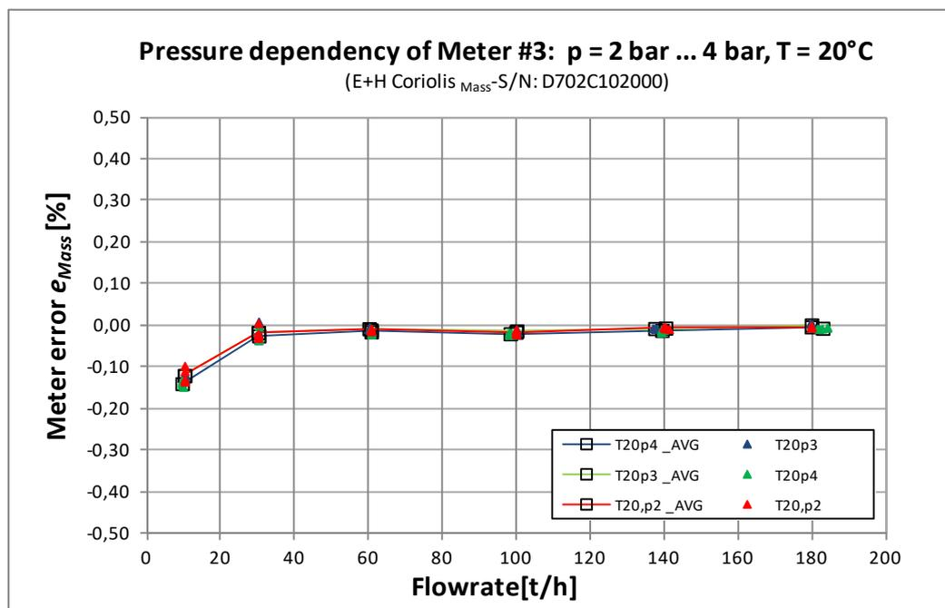
**Figure 18:** Pressure dependency of **Meter #3** (Coriolis<sub>Mass</sub>), measured at PTB in March and April 2013, line pressure: 2 bar, 3 bar and 4 bar, fluid temperature: 20 °C
