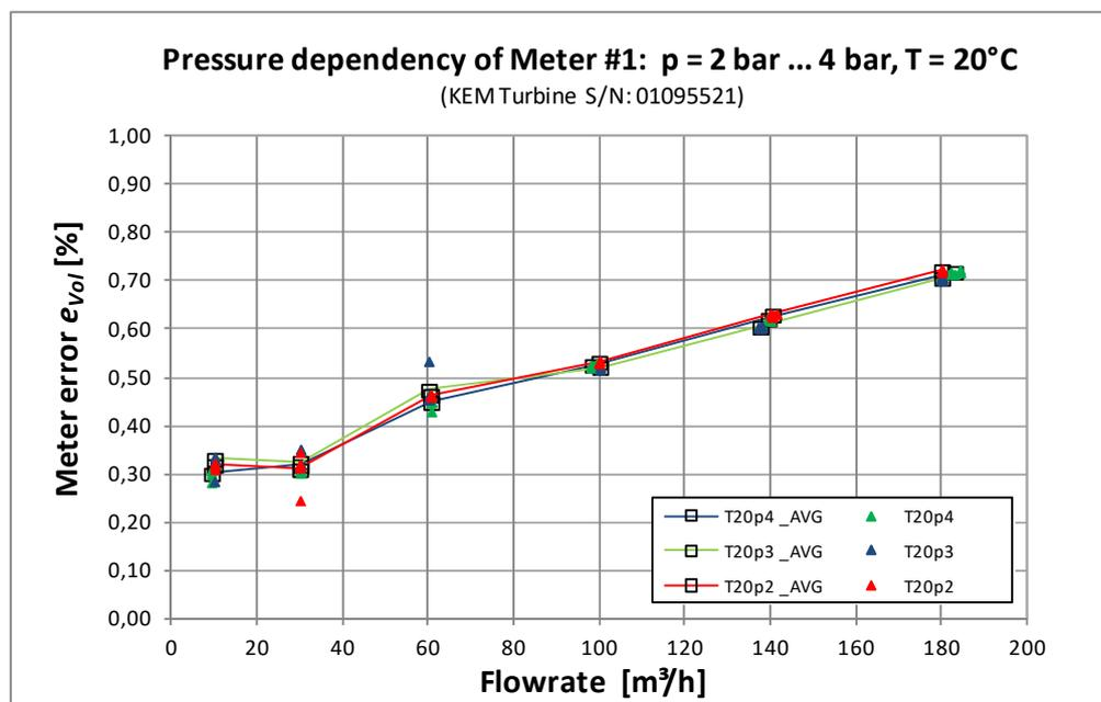
**Figure 14:** Pressure dependency of **Meter#1** (Turbine, KEM), measured at PTB in March and April 2013, line pressure: 2 bar, 3 bar and 4 bar, fluid temperature: 20 °C
