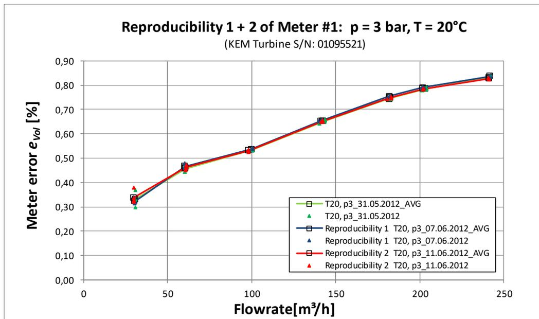
**Figure 21:** Internal reproducibility 1 and 2 of **Meter #1** (Turbine) measured at PTB in May and June 2012 (line pressure: 3 bar, fluid temperature: 20 °C)
