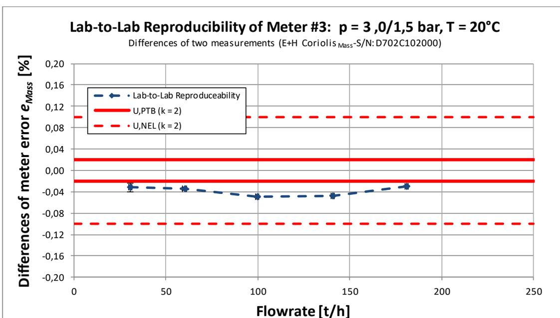
**Figure 32:** Lab-to-Lab reproducibility of **Meter #3** - Differences of measurement error data (17.04.2012 vs. 31.05.2012) of Figure 31 including error bars of maximum standard deviation for one of the comparison pairs
