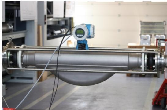
**Figure 5:** Coriolis meter (**Meter #3**)
