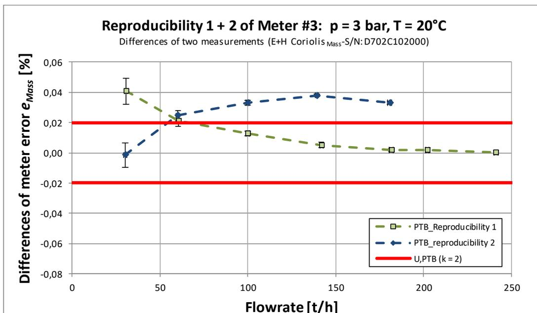
**Figure 26:** Internal reproducibility 1 and 2 of **Meter #3** - Differences of measurement error  $e_{Mass}$  for repeatability data (07.06.2012 vs. 31.05.2012) and for reproducibility data (02.04.2013 vs. 07.06.2012) of Figure 25 including error bars of maximum standard deviation for one of each pairs
