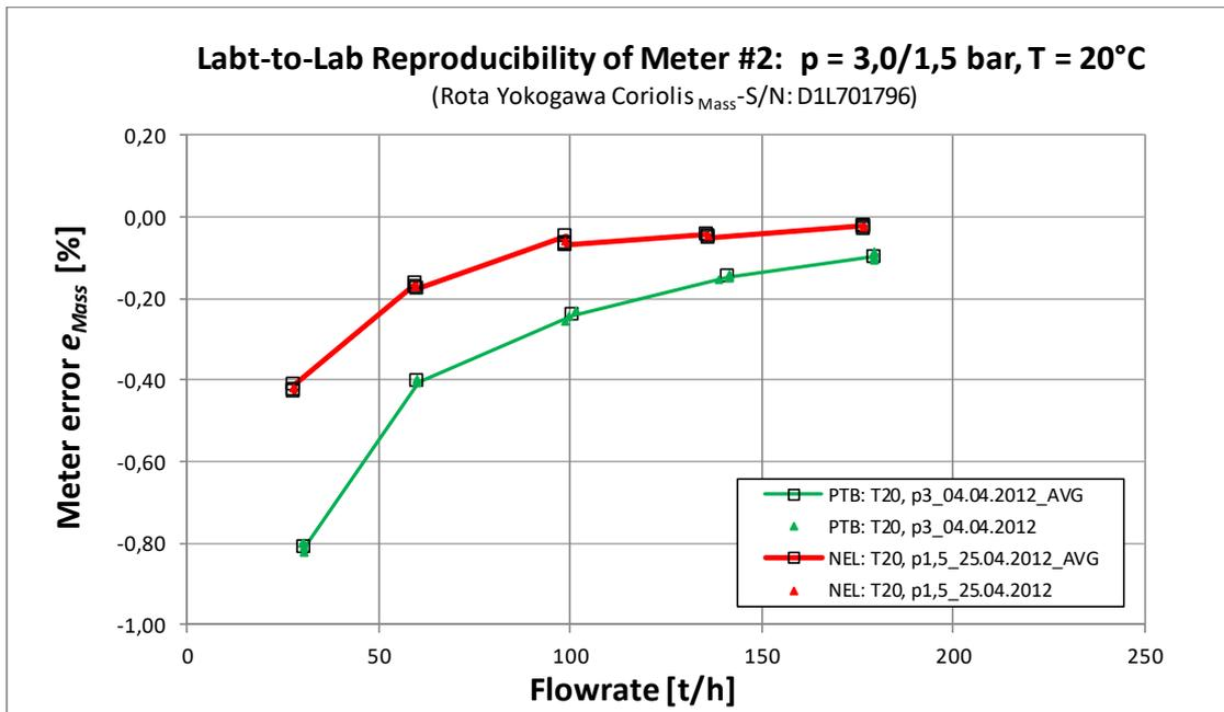
**Figure 29:** Lab-to-Lab reproducibility of **Meter #2**, measured at PTB on 04.04.2012 and at NEL on 25.04.2012. Fluid temperature  $20^{\circ}\text{C}$  (both at PTB and NEL), line pressure: 3,0 bar at PTB and 1,5 bar at NEL. K-factor: 144 pulses/kg (both at PTB and NEL).
