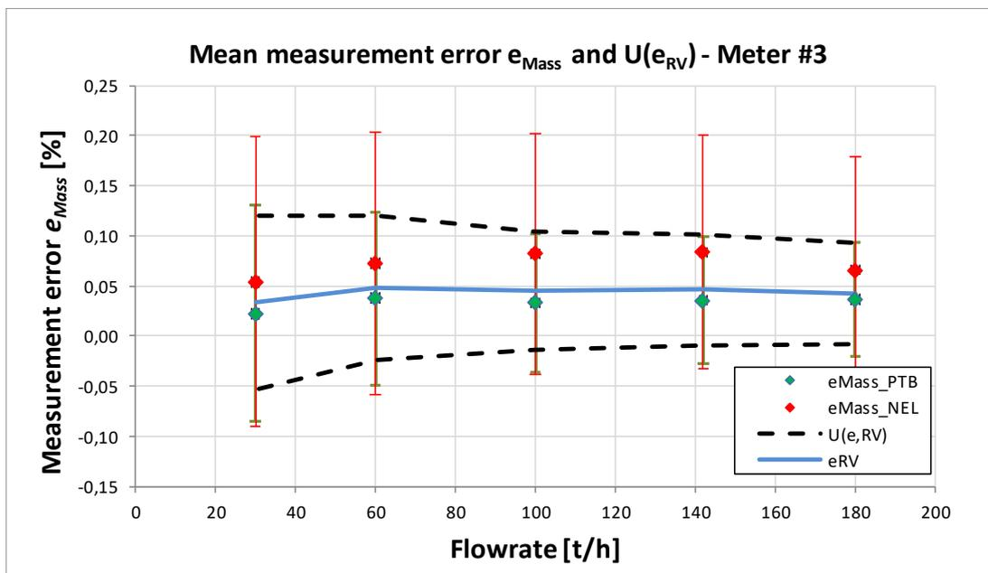
**Figure 38:** Measurement error of  $\bar{e}_{Vol}$  with error bars  $U(\bar{e}_{Mass})$  for PTB and NEL of **Meter #3**. reference value  $e_{RV}$  and the area of the extended uncertainty of the reference value  $U(e_{RV})$  – for **Meter #2**
