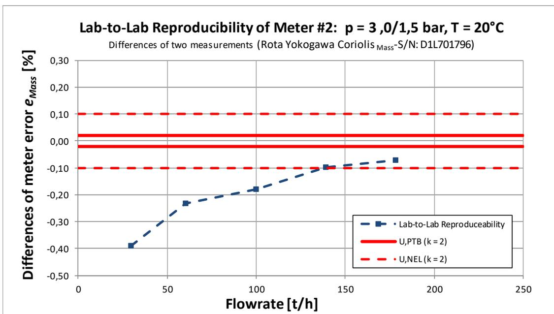
**Figure 30:** Lab-to-Lab reproducibility of **Meter #2** - Differences of measurement error data (25.04.2012 vs. 04.04.2012) of Figure 29 including error bars of maximum standard deviation for one of the comparison pairs
