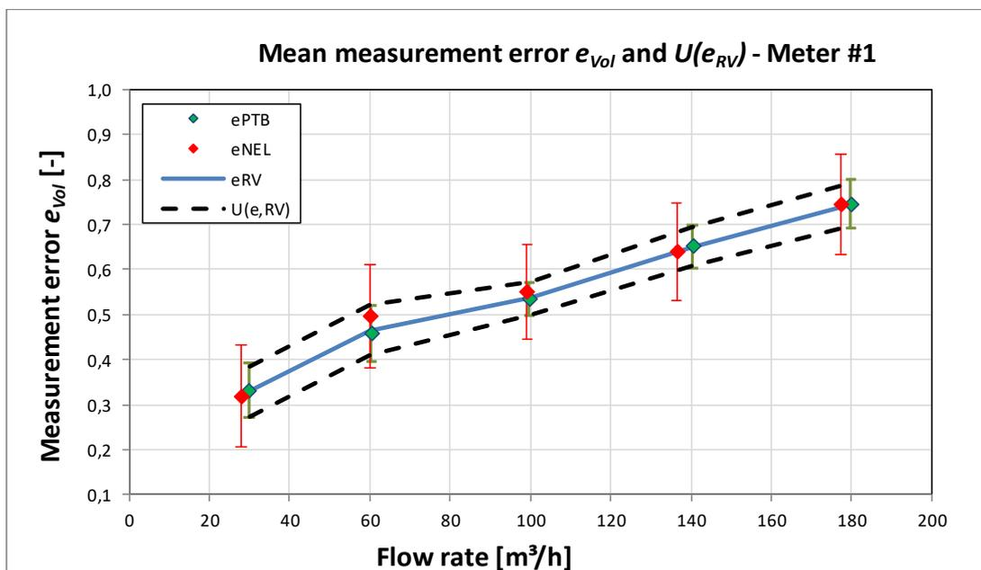
**Figure 34:** Measurement error of  $\bar{e}_{Vol}$  with error bars  $U(\bar{e}_{Vol})$  for PTB and NEL of **Meter #1**. reference value  $e_{RV}$  and the area of the extended uncertainty of the reference value  $U(e_{RV})$  – for **Meter #1**
