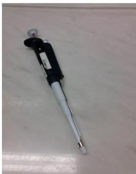
**Figure 1- variable micropipette of 1000 µl**
