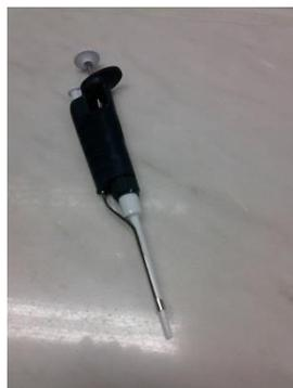
**Figure 2- variable micropipette of 100 µl**
