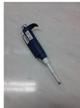
**Figure 4- variable micropipette of 2 µl**
