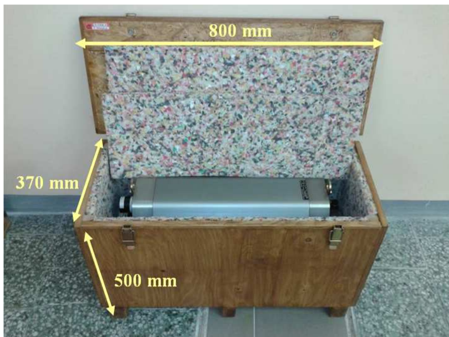
Figure 5 – The wooden box for the rotary piston gas meter G650
