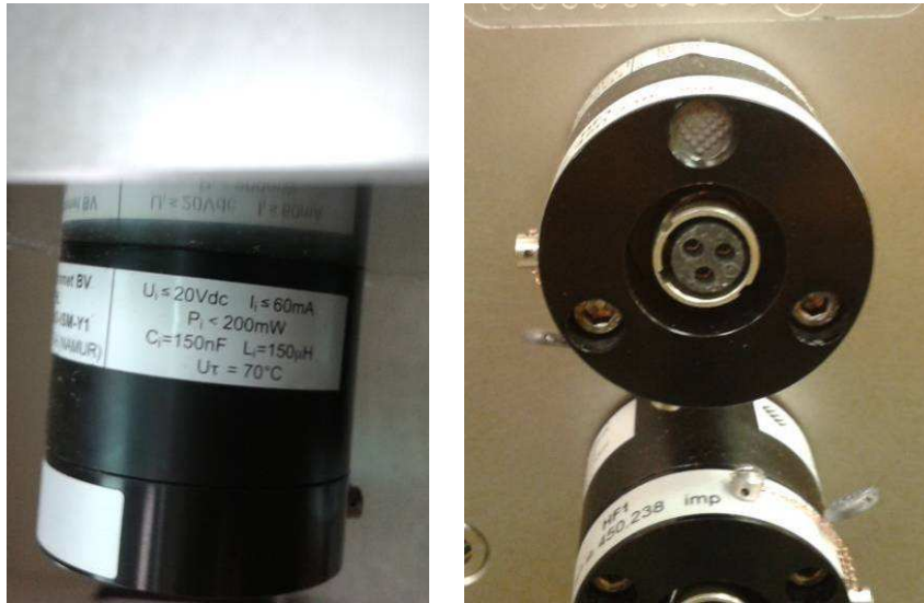
Figure 3 – HF pulse emitter REPROX
