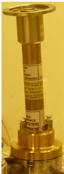
Figure 2. A transfer standard on its base with the trim masses added. Figure 3. Photograph of the utilized mass comparator.
