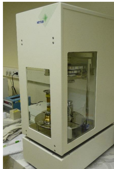
Figure 2. A transfer standard on its base with the trim masses added. Figure 3. Photograph of the utilized mass comparator.
