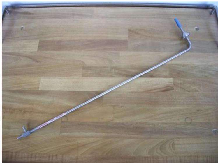
Figure 3-2 Special amplified Pitot tube (secondary Instrument).
