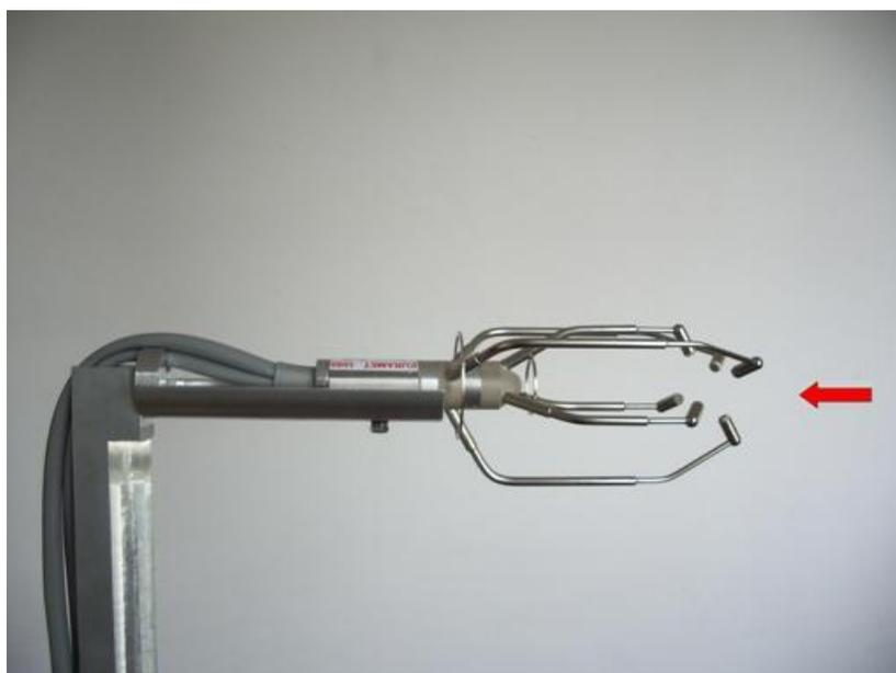
Figure 3-1 Ultrasonic Anemometer sensing element; the arrow indicates the flow direction.
