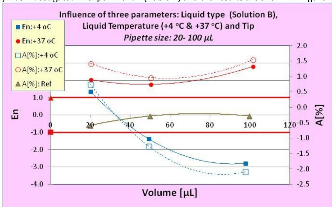
Figure 16. Simultaneous influence of liquid type, liquid temperature and tip type on medium size pipettes
