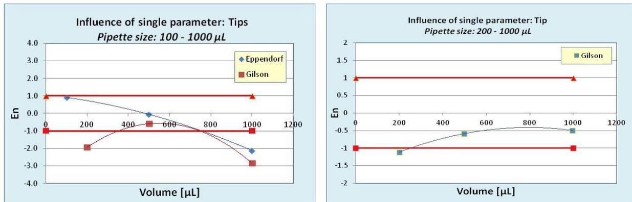
Figure 5. Influence of tip type in medium and large size pipettes
