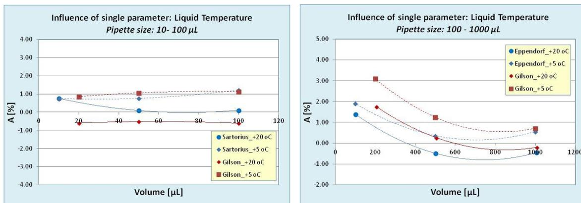
Figure 11. Influence of H<sub>2</sub>O temperature on the accuracy of the delivered volume (quantitative)
