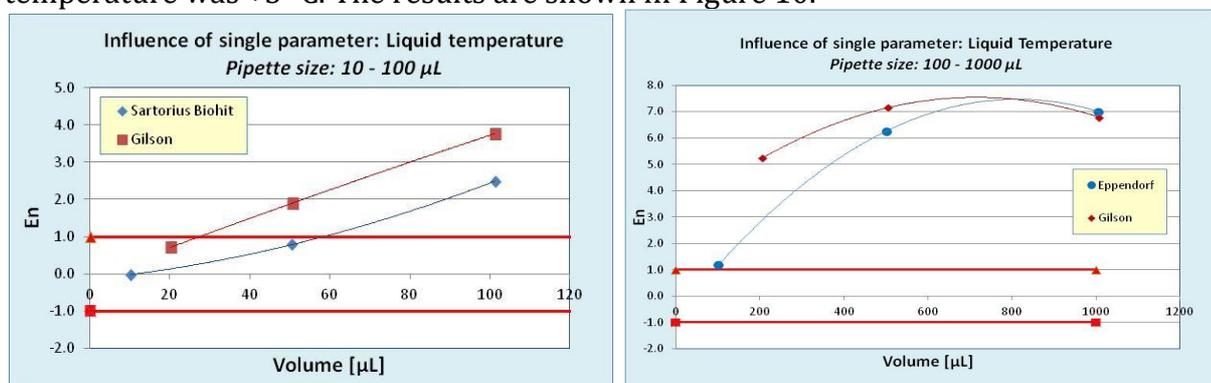
Figure 10. Influence of  $\text{H}_2\text{O}$  temperature in medium and large size pipettes (qualitative)
