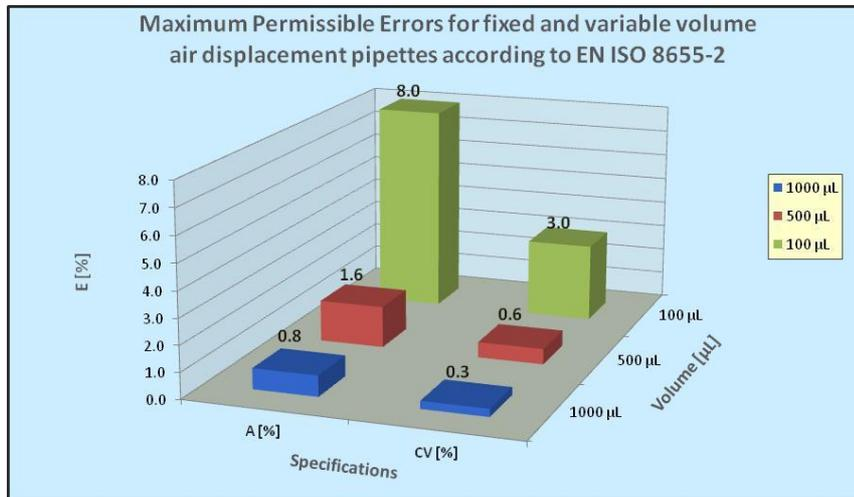
Figure 4. EN ISO 8655-2 specifications for 100 – 1000 µL variable volume pipettes. The evaluation, however, of the obtained results in the present investigation was done on a **qualitative** and a **quantitative** basis according to the criteria given in Figure 5.
