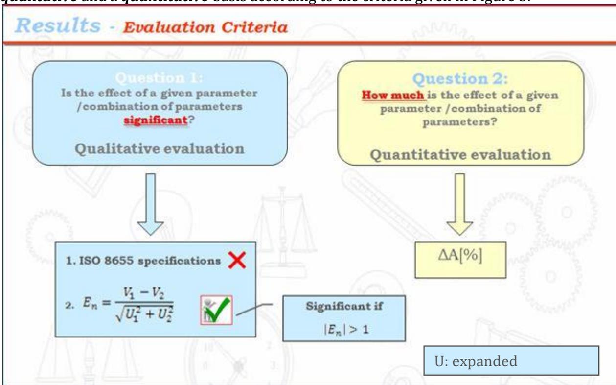
Figure 5. Evaluation criteria for the interpretation of the results. The ISO 8655 specifications were not chosen to be the criterion for the evaluation because they are considered to be too high and modest for this type of investigation. Applying this type of evaluation the results obtained during the course of this project are presented graphically in the next paragraphs categorized in two main groups:
