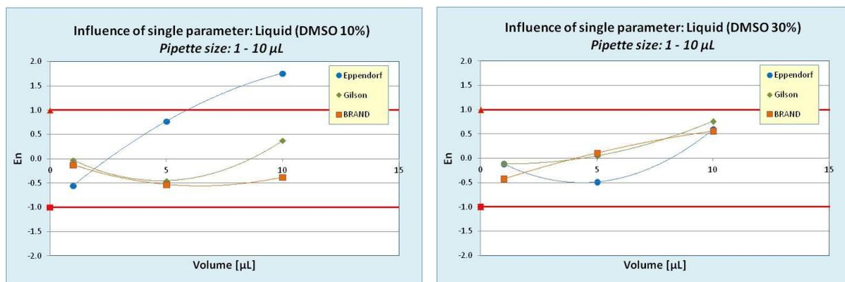
Figure 8. Influence of liquid type (10% & 30% DMSO solutions) in small pipettes of three different manufacturers
