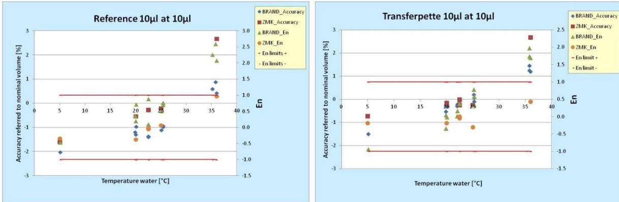
Figure 17. Influence of H<sub>2</sub>O temperature at 10 µL
