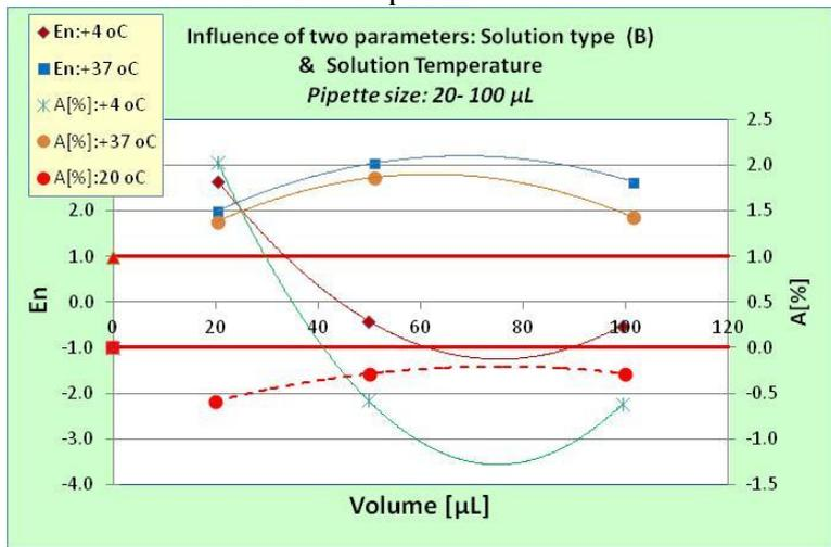
Figure 13. Combined influence of liquid type and temperature on medium size pipettes
