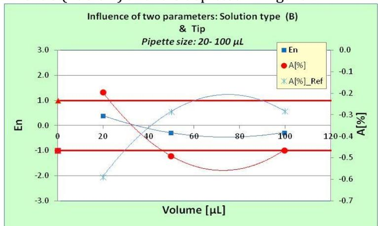
Figure 14. Combined influence of liquid type and tip on medium size pipettes
