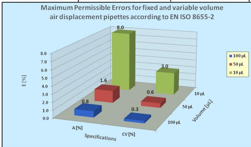
Figure 3. EN ISO 8655-2 specifications for 10 – 100  $\mu\text{L}$  variable volume pipettes
