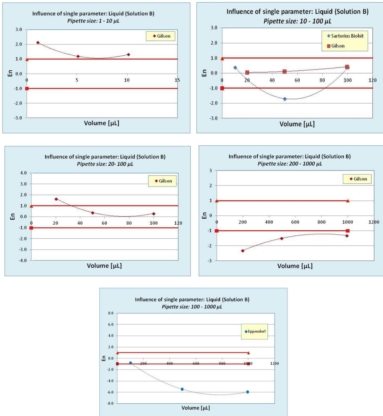
Figure 7. Influence of liquid type (Solution B) in small (1-10 µL), medium (10-100 µL/20-100 µL) and large size (100-1000 µL/ 200-1000 µL) pipettes
