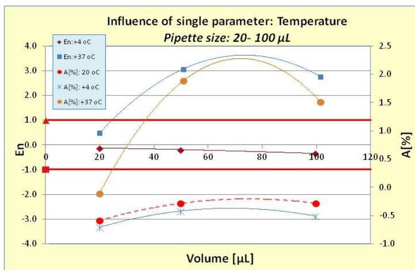
Figure 12. Influence of H<sub>2</sub>O temperature in medium size pipettes
