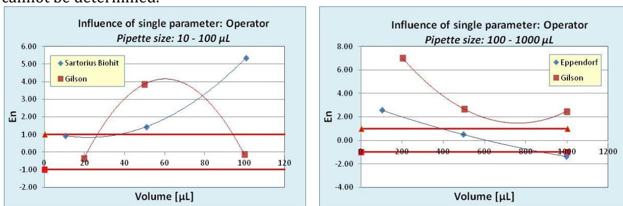
Figure 6. Influence of operator in medium and large size micropipettes
