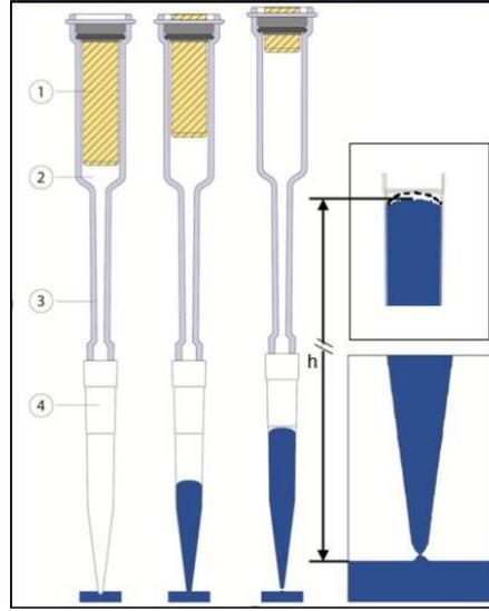
Fig. 1 Aspiration of a liquid using an air cushion pipette: (1) piston, (2) captive air, (3) shaft, (4) tip, while h denotes liquid lift in the tip (by courtesy of BRAND GMBH +CO KG).
