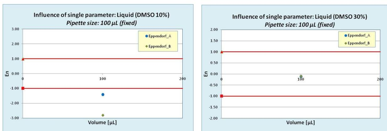
Figure 9. Influence of liquid type (10% & 30% DMSO solutions) in fixed volume 100  $\mu\text{L}$  pipettes of the same manufacturer
