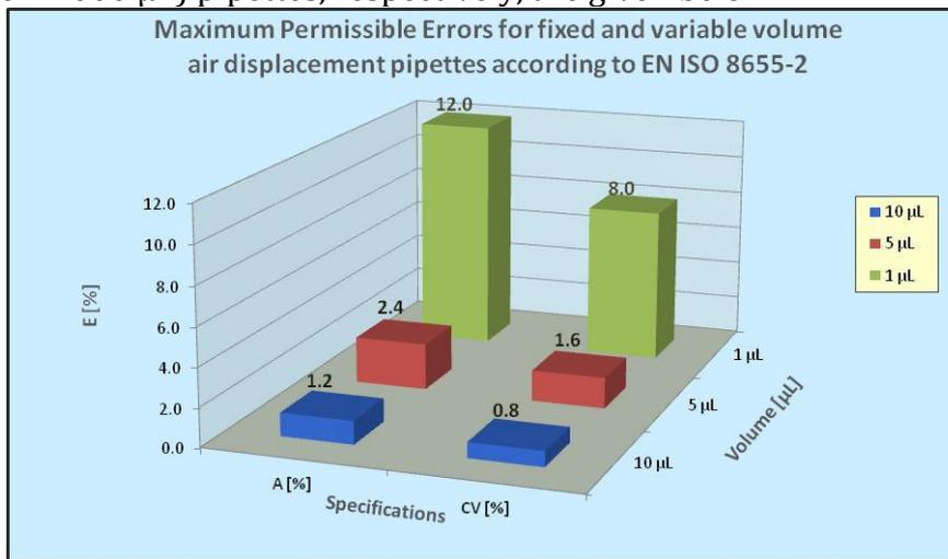
Figure 2. EN ISO 8655-2 specifications for 1 – 10  $\mu\text{L}$  variable volume pipettes
