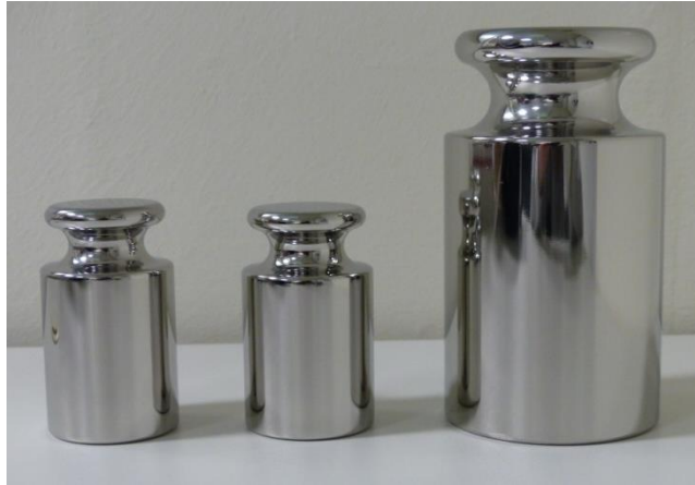
Figure 1: Photograph of the first three transfer standards used for this intercomparison: 1 kg-knob weight with flat bottom (marking “Z2”) on the left, 1 kg-knob weight with recessed base in the middle and 5 kg-knob weight with flat bottom (marking “5 kg”) on the right.
