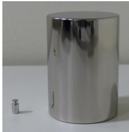
Figure 2: Photograph of the two other weights used for this intercomparison: 2 g-knob weight with recessed base on the left and 1 kg-hollow cylinder (marking “•”) on the right.
