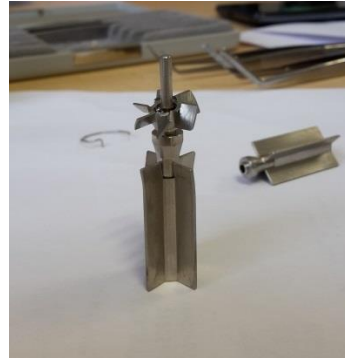
Figure 1 - Photos of the broken FT-12 turbine
