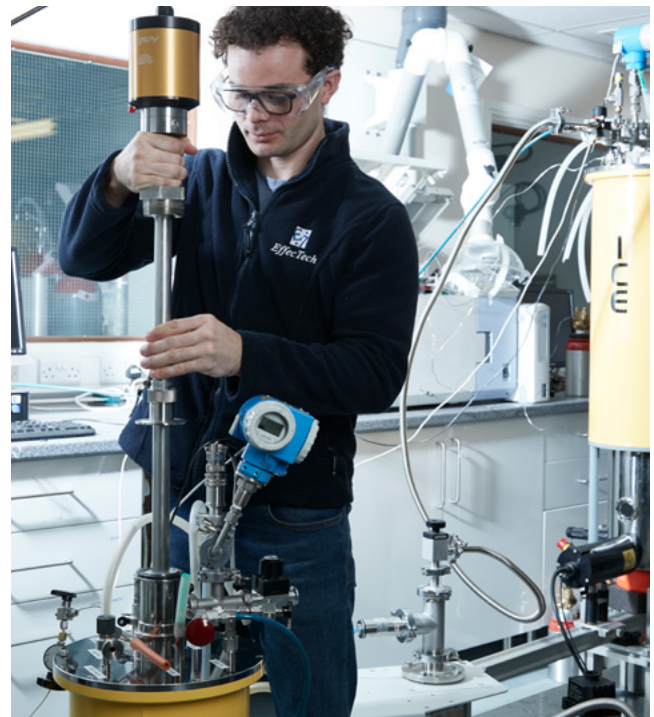
Dr Joey Walker inserting the LNG probe into the custom-built EffecTech liquefier
