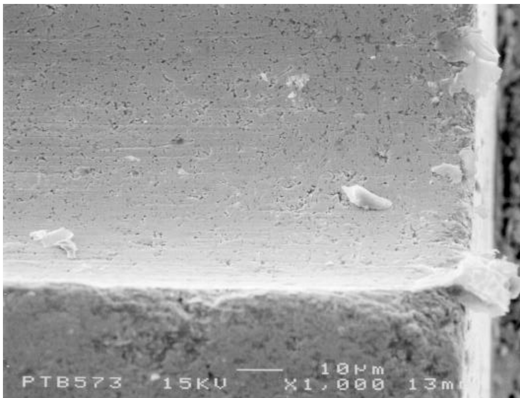
Figure 26: REM shot of a cut ring gauge (0,1 mm in diameter), detail
