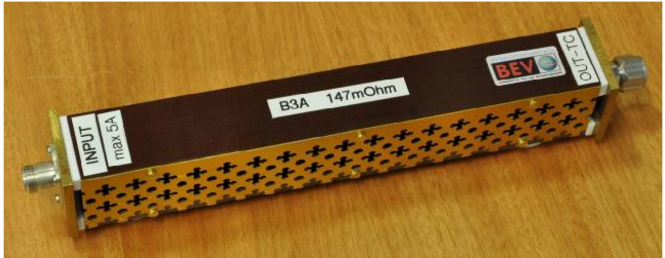
Figure 2: Physical layout of the 5A travelling standard
