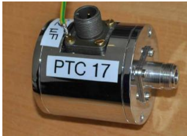
Figure 1: Physical layout of the 10 mA travelling standard
